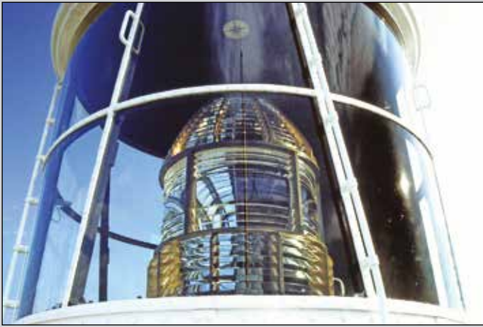
Third order fixed optic at Cromer lighthouse, 1987. Photo by Trevor Haywood
